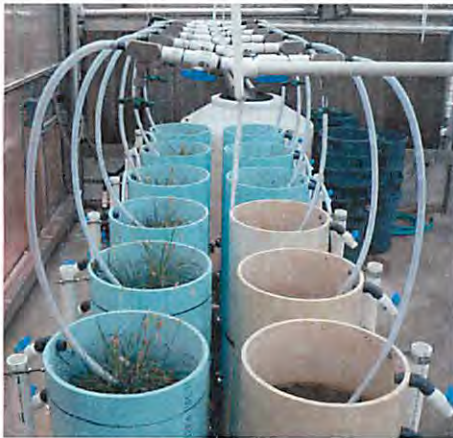
Figure 1. Large bioretention columns at Washington State University in Puyallup, WA used to test biological effectiveness of bioretention.
